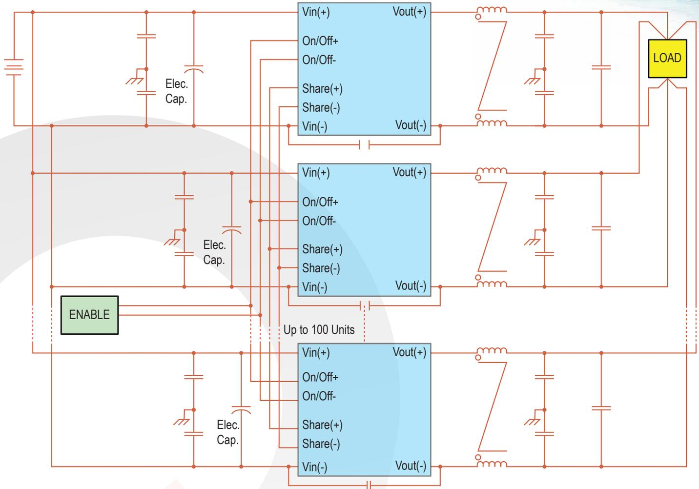
Figure G: Typical Application Circuit for Paralleling of Full-Featured Units with an Output Common-Mode Choke. See Figure F for configuration with an input common-mode choke.
