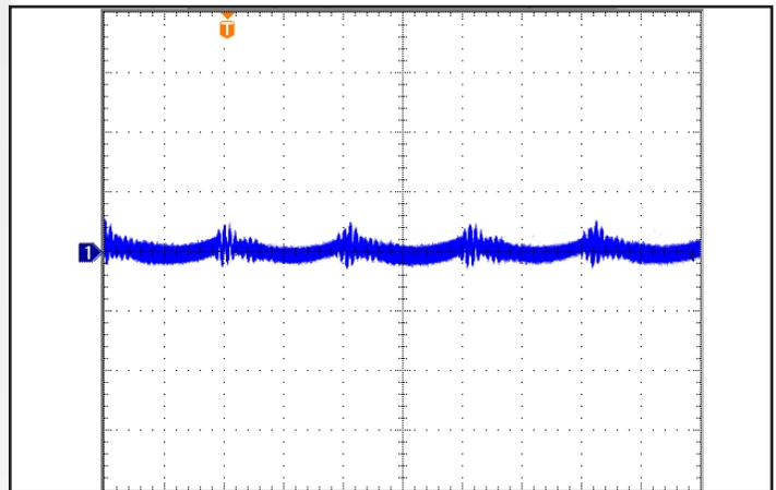
**Figure 10:** Output voltage ripple at nominal input voltage and rated load current. Output capacitance: 100µF electrolytic in parallel with 1µF ceramic. Ch1: Vout (200 mV/div; BW= 20MHz). Horizontal Scale: 2µsec/div.
