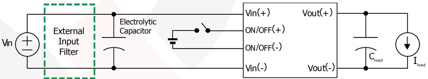
Figure D: Typical Application Circuit (negative logic unit, permanently enabled)
