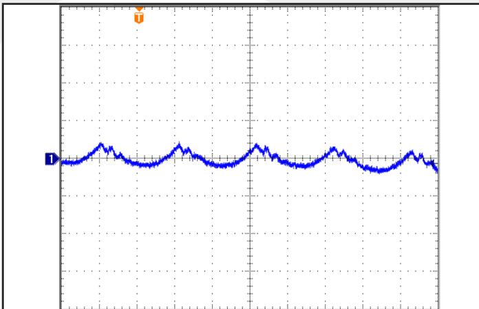
**Figure 9:** Input terminal current ripple at full load and nominal input voltage. Output capacitance: 100µF electrolytic in parallel with 1µF ceramic. Ch 1: Input (1.0A/div; BW= 20MHz). Horizontal Scale: 2µsec/div.
