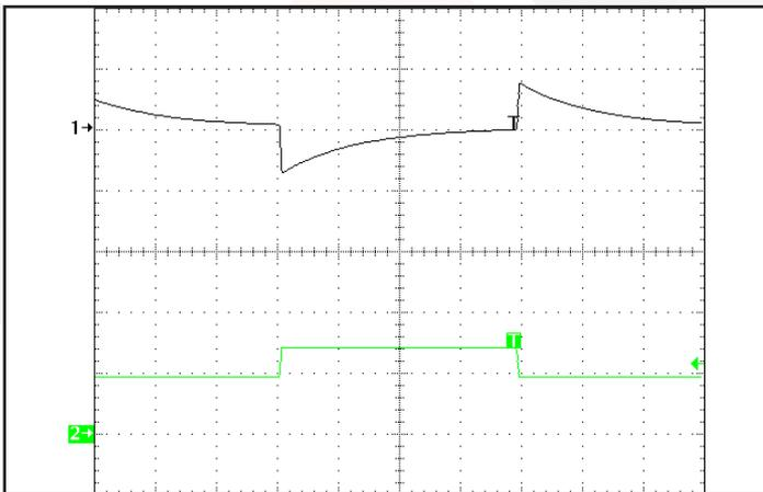
**Figure 11:** Output voltage response to step-change in load current (50%-75%-50% of Iout(max); dI/dt = 0.1 A/µsec). Output capacitance: 100µF electrolytic in parallel with 1µF ceramic. Ch 1: Vout (5V/div), Ch 2: Iout (2A/div). Horizontal Scale: 100msec/div
