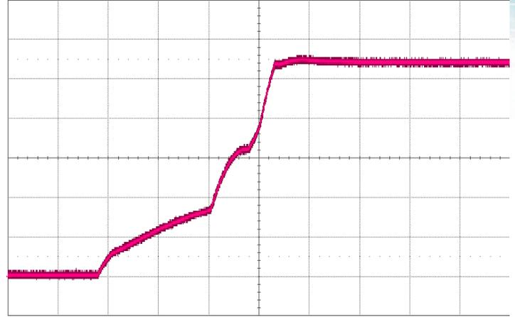
Figure 8: Output voltage startup waveform with 400 $\mu$ F hold-up capacitor, no load (115VAC, 60Hz), (50V/div), Timebase: (500ms/div)
