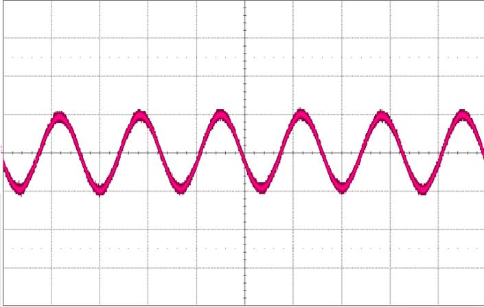
Figure 7: Output voltage ripple with 400 $\mu$ F Hold-up capacitor at full rated power (115VAC, 60Hz)  $V_{out}$  (5V/div), Timebase: (5ms/div)
