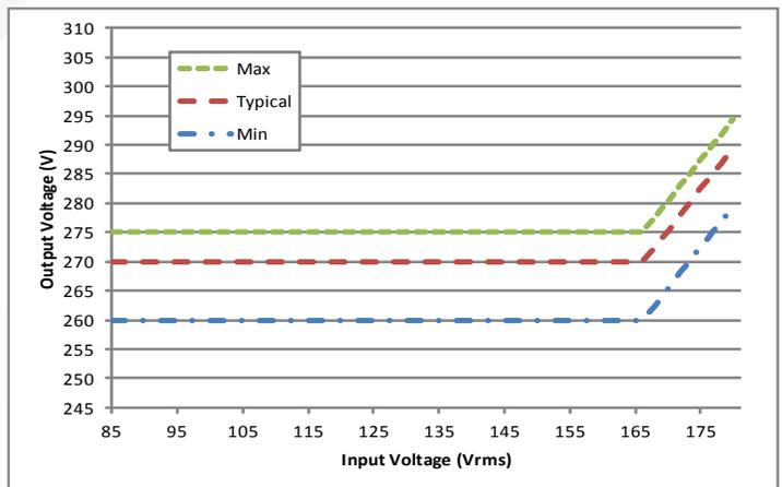
Figure 6: DC output voltage range vs. input voltage
