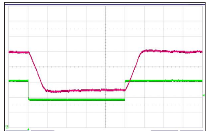
Figure 12: Output Current vs Iset pin voltage dynamics; 28Vin 10Vout (5mS/div). Top Trace: Output Current (2A/div). Bottom Trace: Iset pin voltage (200mV/div).
