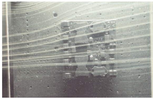
Figure 11b: Airflow over SynQor converter showing free flow of air over the converter
